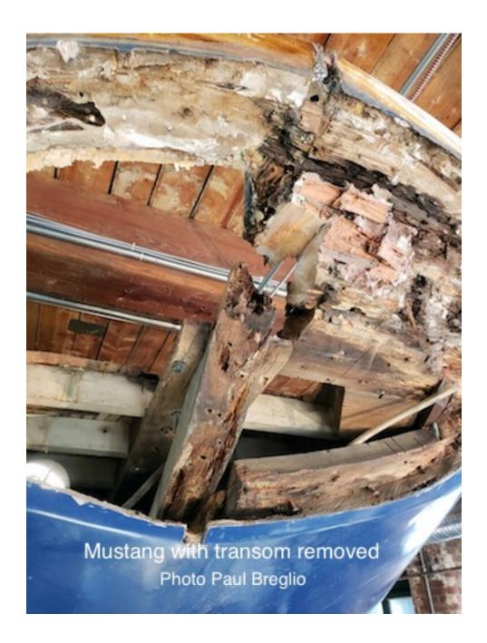
Breglio wrote (em 4/19) after working to open up the areas of concern that " deck leaks were mostly confined to the aft near the taftrail and around the mast opening. I am in the process of removing all of the stanchion bases where there was leakage as well. The entire transom was rotted under the fiberglass skin due to a compromised seal where the glass met the taftrail. Much
